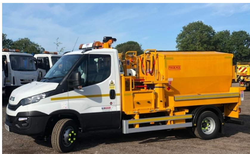
Hot-Box Pothole Repair Vehicle.
